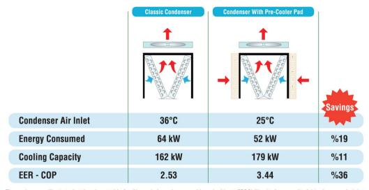
The savings are illustrated at the above table for Air cooled condensers with and without FESChill unit. As a result of 11c decrease in inlet air, the energy consumed by the Chiller is decreased by 19 % and the cooling capacity is increased by 11 %. This allows the EER or COP of the chiller to increase by 36 %. On average every 1.8c decrease of air inlet temperature achieved by the pre-cooling pads, increases the condenser effectiveness by 2 %.
