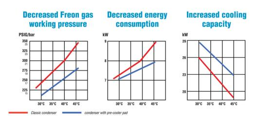
The cooler air inlet decreases the system working pressure, which creates increased cooling capacity and decreased energy usage.
